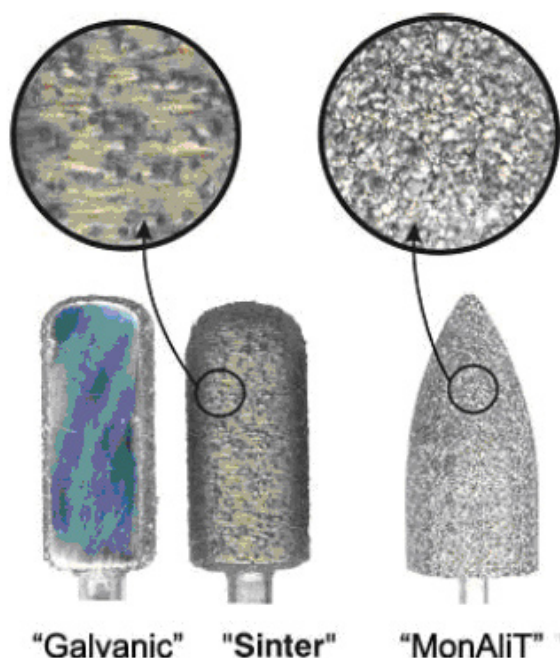
Fig.1. Comparison in diamonds quantities between “Galvanic”, “Sinter” and “MonAliT” tools.
